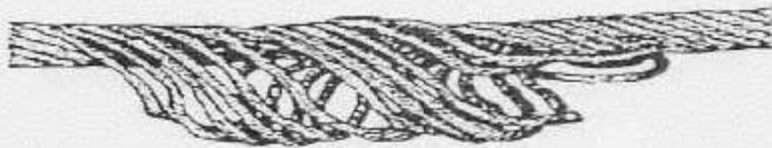
D THIS IS A TYPICAL BIRD CAGE CONDITION.
