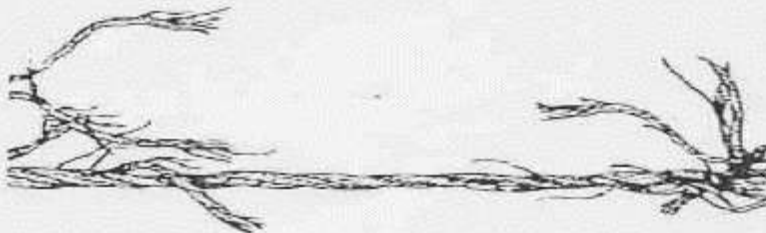
E THIS IS THE APPEARANCE OF A TYPICAL TENSION BREAK: A RESULT OF OVERLOADING.
