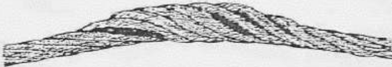
E THIS EFFECT OF DRUM CRUSHING IS EVIDENCE OF BAD WINDING CONDITIONS.
